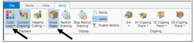
4. Click on **File>Options** and then on the **General** menu, enable **Collision Checking** with the **Tool to the Fixture**. Click **Ok**.
