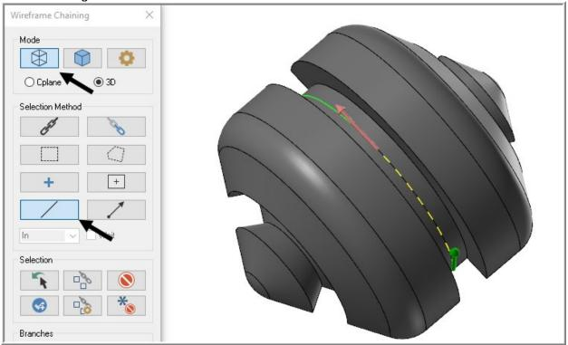
6. The **Tool Axis Control** will be left to **Surface**. Click the selection button and select the face under the previously selected wireframe arc. Click **End**.
